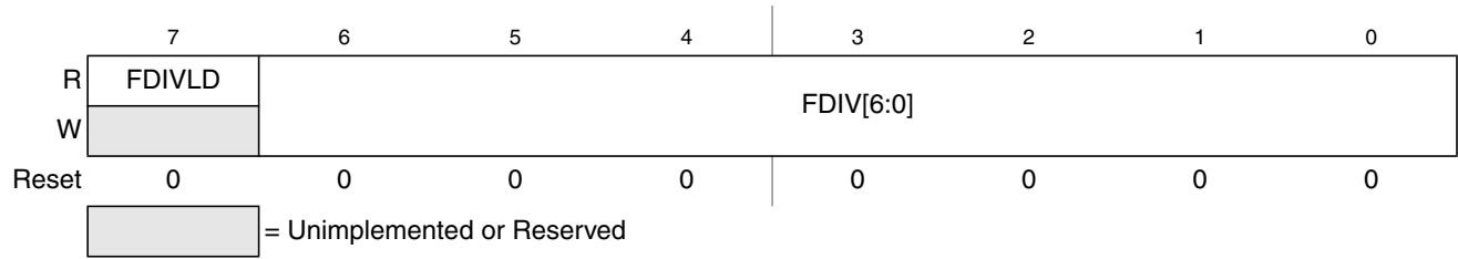
Figure 29-5. Flash Clock Divider Register (FCLKDIV)
