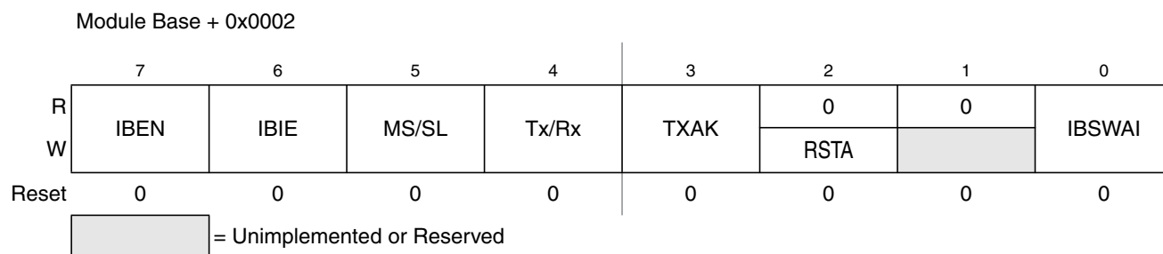
Figure 15-6. IIC Bus Control Register (IBCR)
