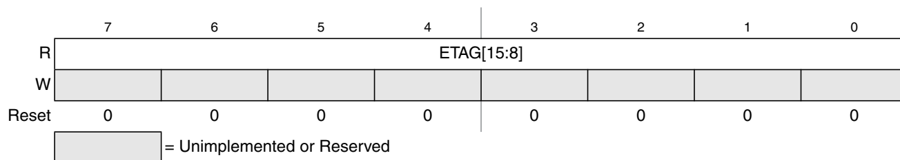
Figure 26-18. EEE Tag Counter High Register (ETAGHI)
