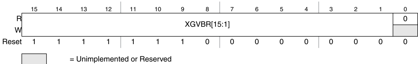
Figure 10-9. XGATE Vector Base Address Register (XGVBR)
